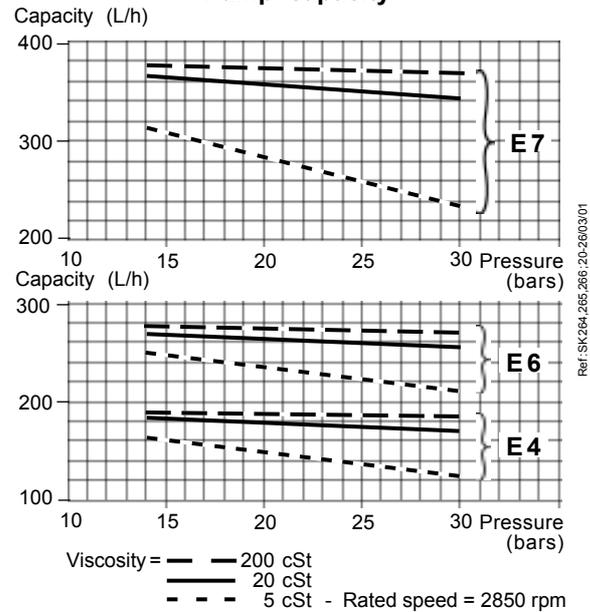
Data shown take into account a wear margin. Do not oversize the pump when selecting the gear capacity.
